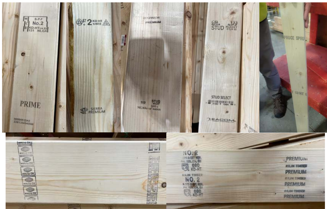
Figure 3 – Shows several examples that illustrate use of ALSC grade terms “Prime”, “Premium”, “Select”, or species on lumber even though these terms may not be in the particular agency’s rule book.
