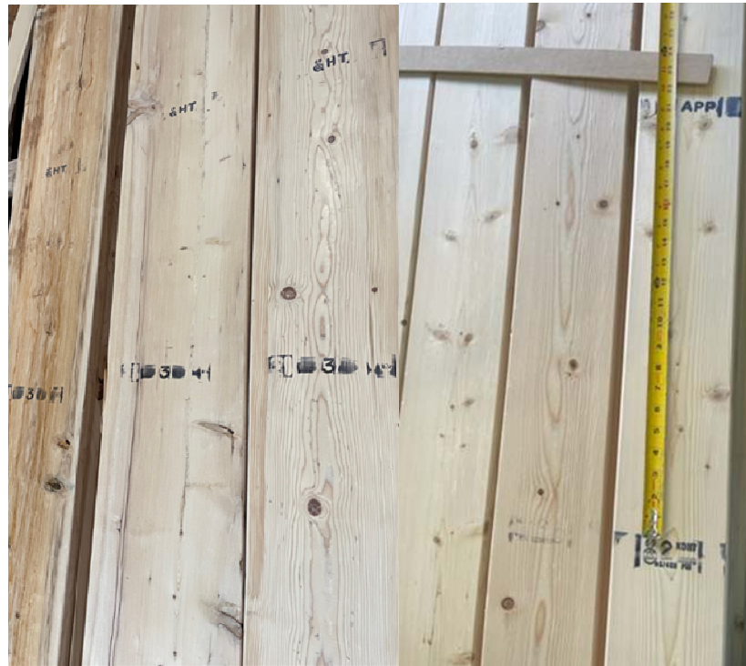
Figure 1 — shows examples of marking grade nomenclature in the applicable accredited agency's rule book even though the boards are not being graded according to the grade designation. The stamped information 3 and APP label are present on lumber when not being graded according to 3 or APP rule.
